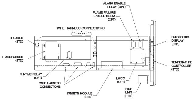
Figure 39 - Control Panel Component Location Drawing
